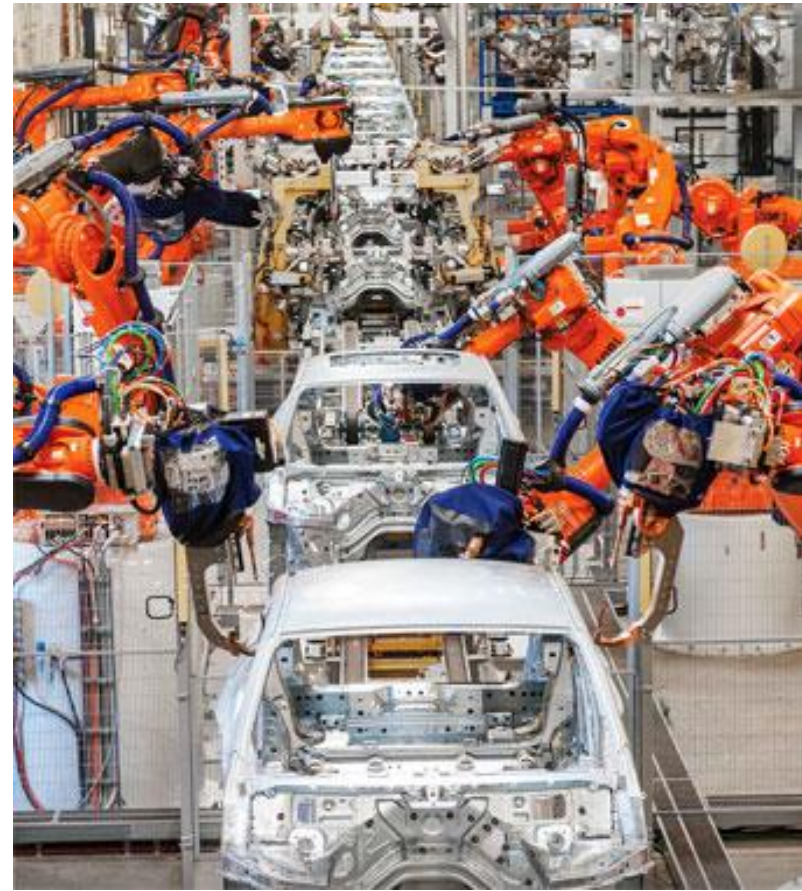
BMW's robotic welding line, in Spartanburg, S.C. [19]
